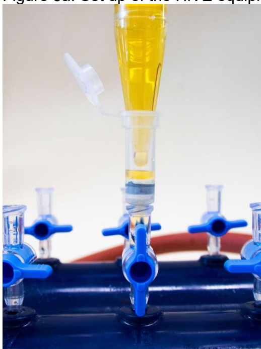
Figure 3b. Close up of the pipette/reservoir, RNA binding column, VacValve and QIAVac vacuum manifold for HiVE.
