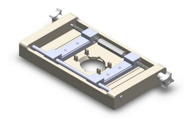
e. Insert the stainless-steel dowel pin (98380A431) through the unthreaded spacer (92320A475) and fix, using glue, the two ends of the dowel pin between the respective holes on top of the base plate. Repeat for the other side.
