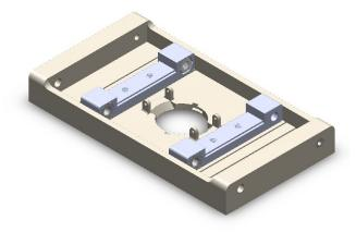
iii. To assemble the lead screw, thread the RH and LH threaded rods from the inside into their respective nuts
