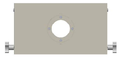
g. Glue the magnetic circular shim within the corresponding indented region of the 3-D printed dish holder. Once the glue is dried, the dish holder should now magnetically attach to the base plate.
