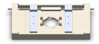
v. Finish assembling the lead screw by attaching an 8-32 thread knob (5993K11) to the outer ends.
