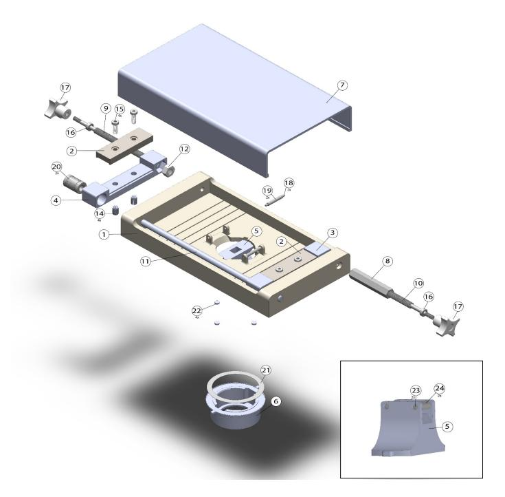
**Figure S2:** Exploded view of the assembled device, with annotation numbers as described in Tables S1 and S2. Since some regions of this device experience high localized stress during tension, the 3-D printed components included structural support features such as side ribs (1) for the base plate and gussets for the indenter (5, in inset).
