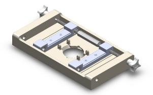
d. Insert the ¼" diameter, 8" long dowel (6061K101) through the opposite ends of the clamp holders. Use glue on the outside to fix the rod in place.
