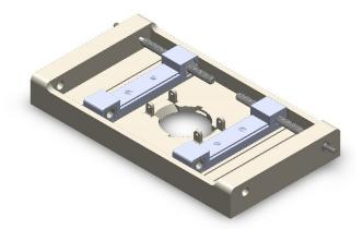
iv. Screw both rods into the LH to RH coupling nut (97372A106) while making sure the clamp holders are centered. After this step, you can test your device by turning the lead screw and making sure that the clamp holders move between the middle and edges of the base plate equidistantly. Only then should you proceed to the next step.
