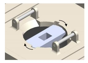
j. When threading a deformable silicone substrate within the device for experiments, screw the clamps into the clamp holders using two M4 12 mm screws (92855A413) per clamp.
