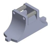
i. To insert the indenter into the base plate, flip over and insert the tabs into the corresponding inserts of the base plate. Twist to lock in place.
